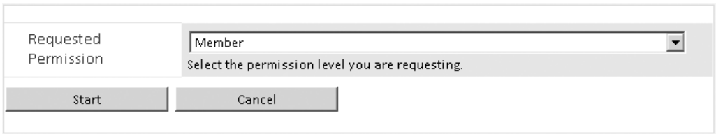
Figure 11-24 The workflow variable you created in SharePoint designer gets converted into a drop-down list allowing the user to select the permission level he or she is requesting
