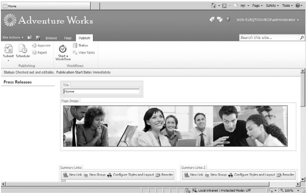
Figure 12-3 Initiating a workflow on a page or pushing out changes for publishing is done with the ribbon functions at the top of the page
